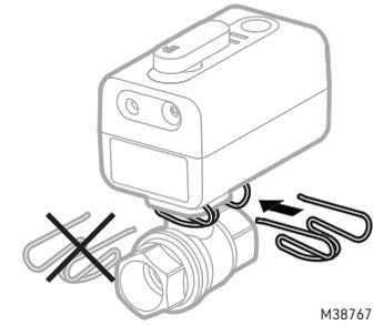
Fig. 4. Connect ball valve to actuator.
